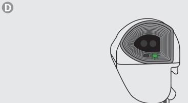
Your device should turn to Normal Operation, System is in Order (green LED flashing).
